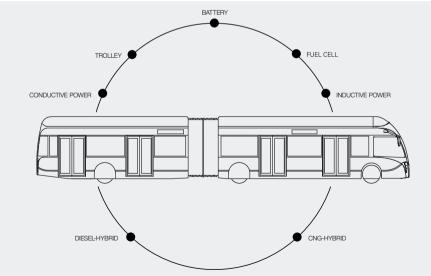
The heart of the Exqui.City is the **Multi Propulsion Platform**, designed to accommodate the latest and greenest alternative propulsion technologies.
